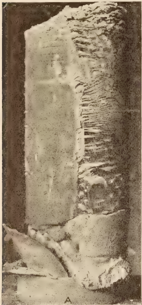
FIGURE 27.—FROZEN CYLINDER, HALF SAND AND HALF CLAY. MUCH SEGREGATED ICE IN CLAY BUT NOT IN SAND. FURNISHED BY TABER EXPERIMENTS
